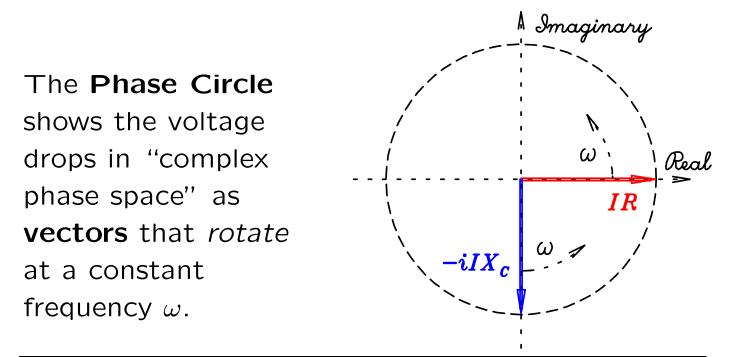
The voltage across the *capacitor* <u>lags</u> behind that across the resistor by an angle of  $\pi/2$ .
